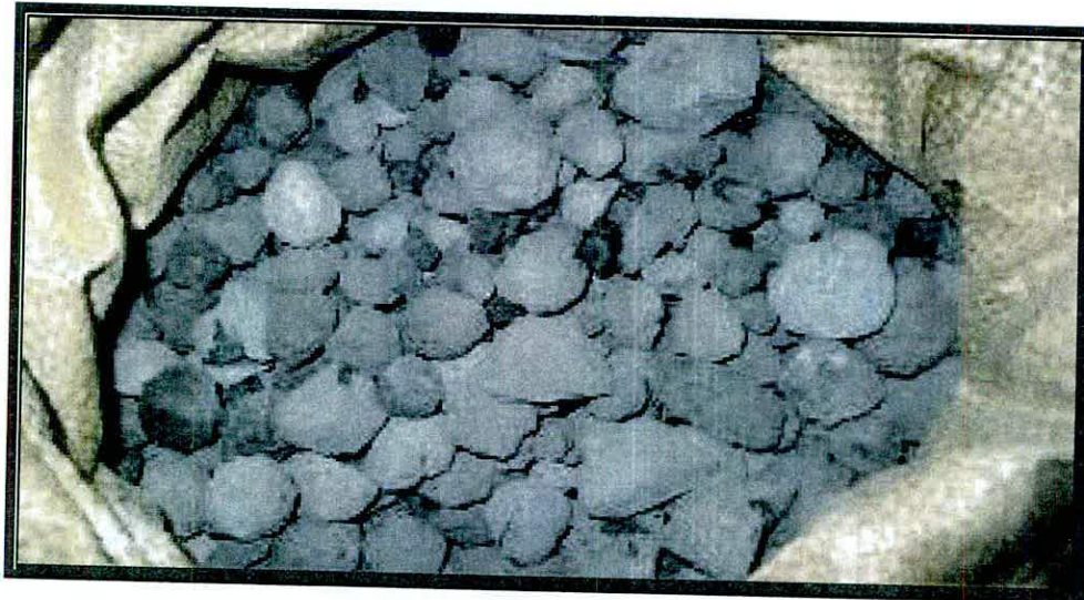
Cooled Clinker from a cooler
