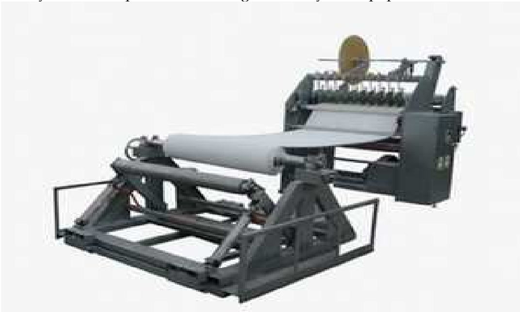
Plaster of Paris bandage slitting and rolling machine POP bandage machine.
