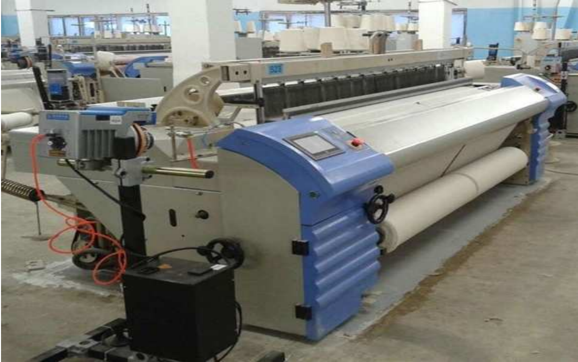
JLH425S medical gauze air jet loom
