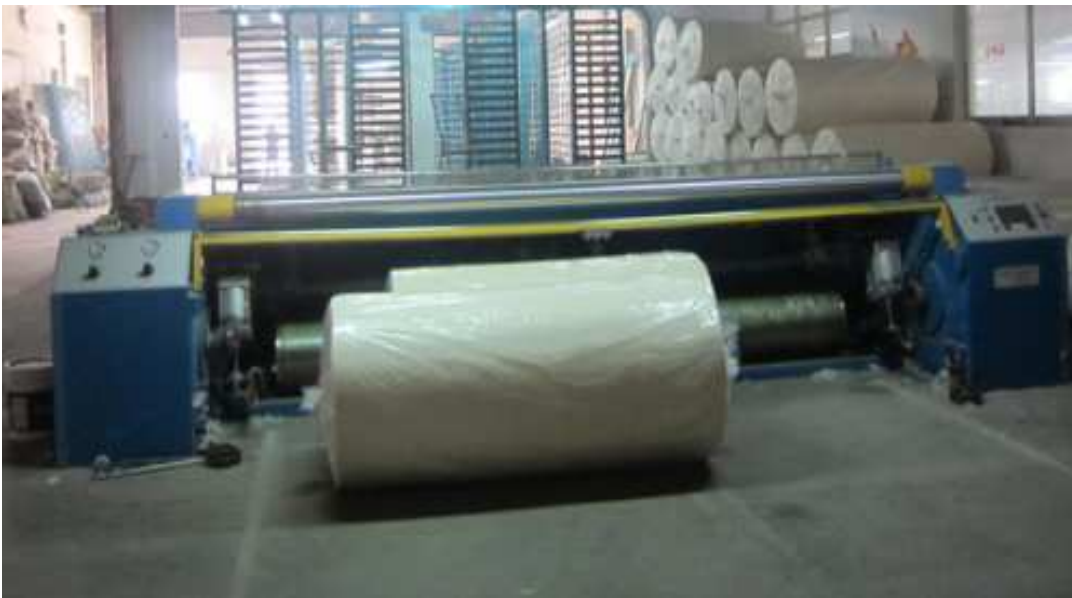
YGA-1 High speed warping machine
