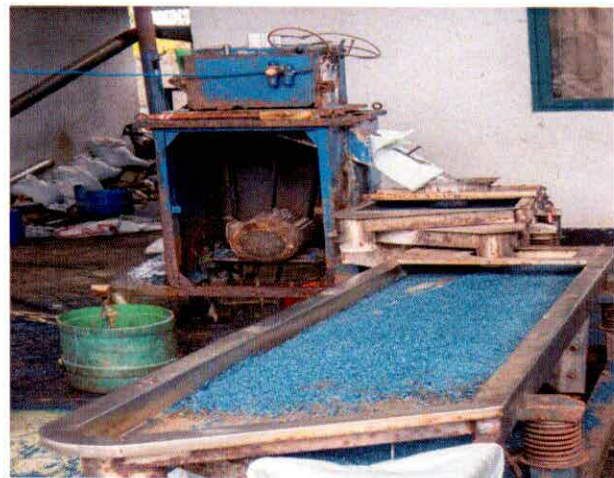
SHREDDING PROCESS (GRANULES AS FINAL PRODUCT)
