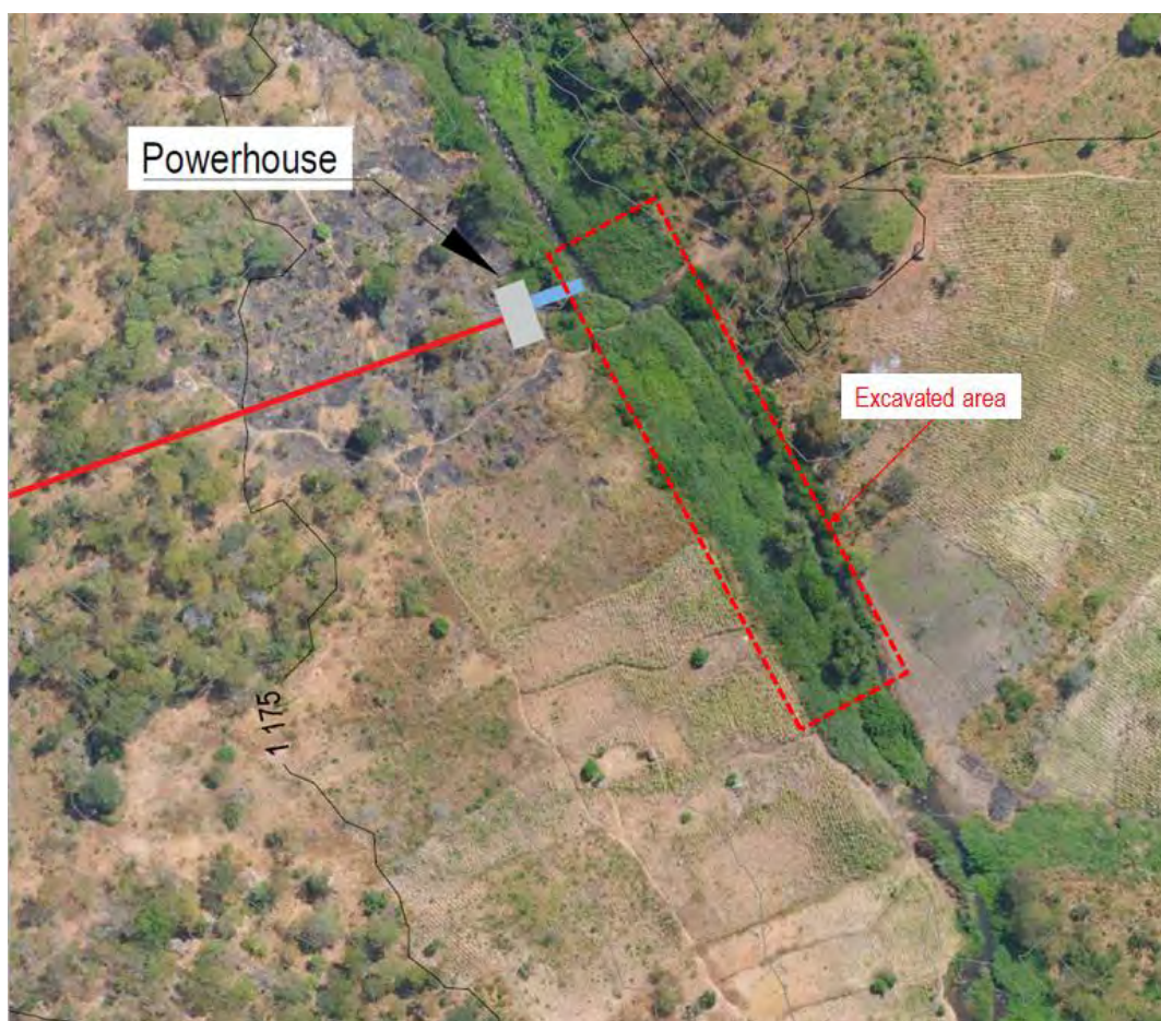
Figure 42. Tailwater zone to be reshaped
