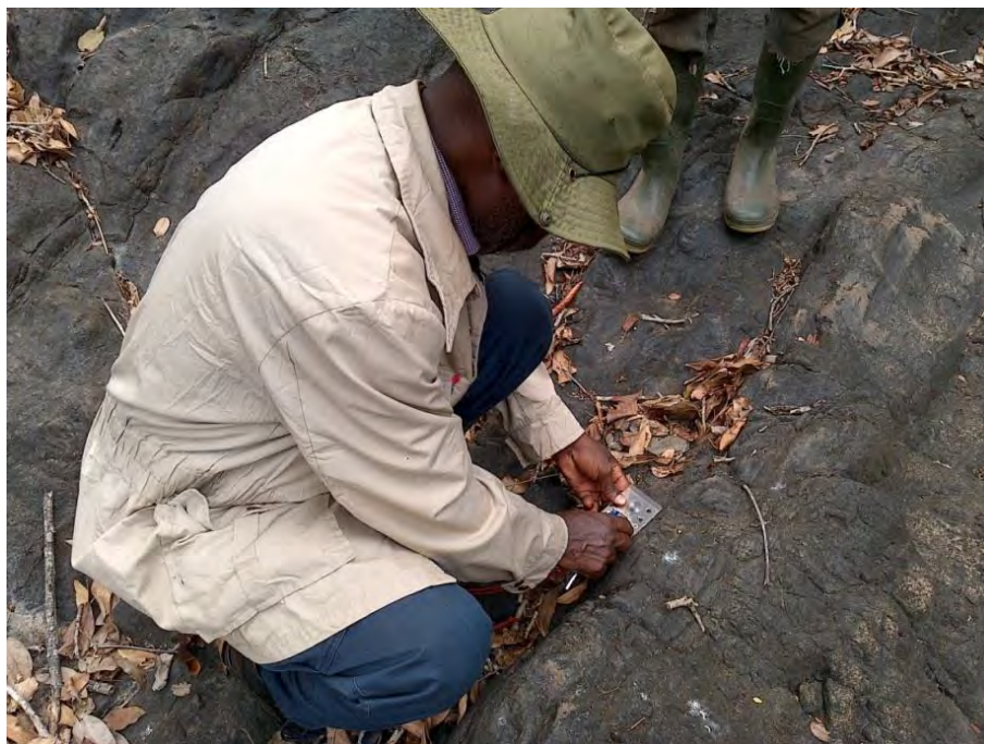
Figure 22. Foliated quartzo-feldspathic gneiss as observed 10m west of the proposed power station
