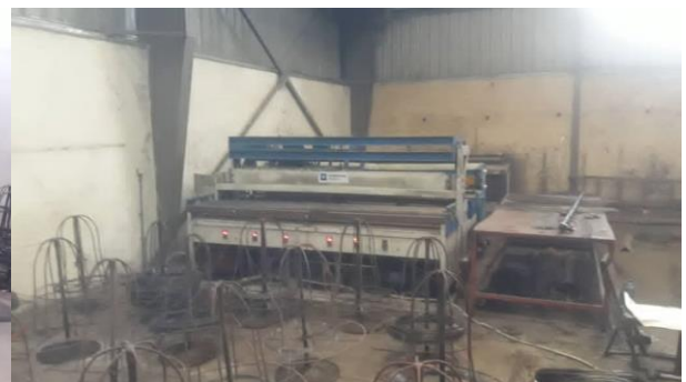
Welded mesh machine
