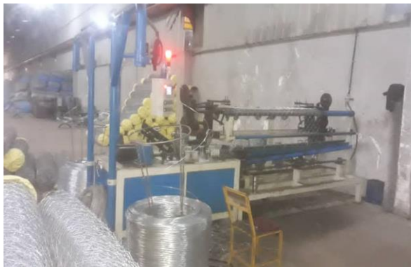
Chain-link fence making machine
