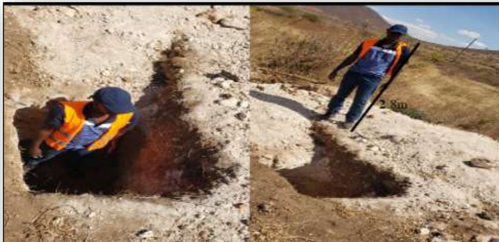
Figure 10. Pit with 2.8 m depth examine physical of limestone deposit at Makalavati Sejeli Hill Limestone
