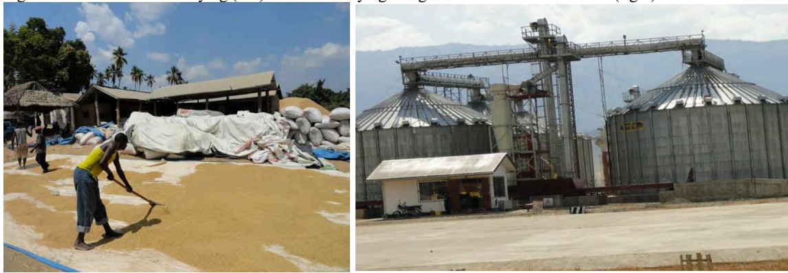
Figure 0.2: Traditional sun drying (left) and hot air drying using rice bran as the heat source (right)
