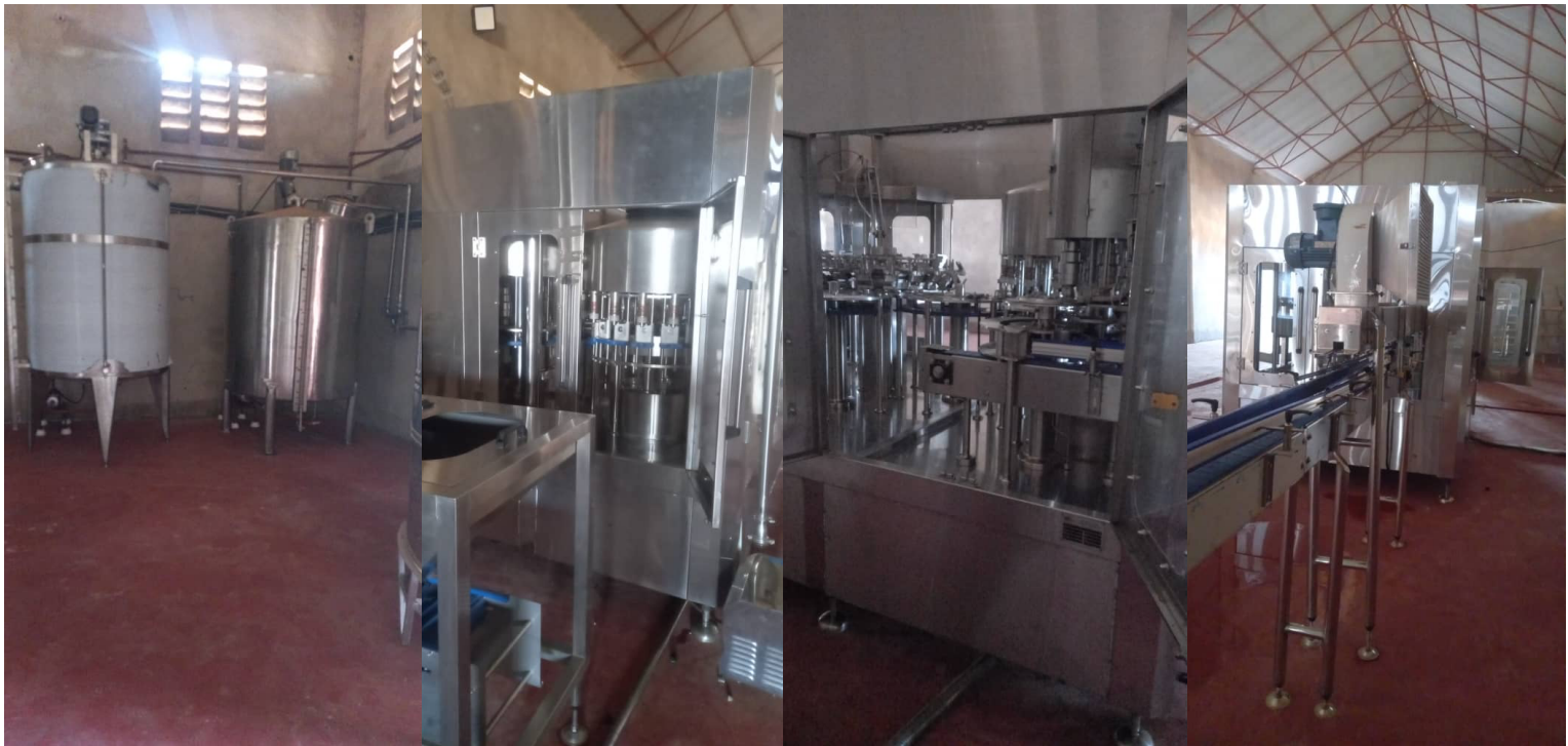
Blending tanks and the Bottle washing , product filling , bottle capping and labelling production plant line. For a capacity of up to 9000 bottles per hour.
