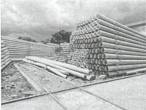
Photo 3: Concrete poles produced at site (Source, PVV team)
