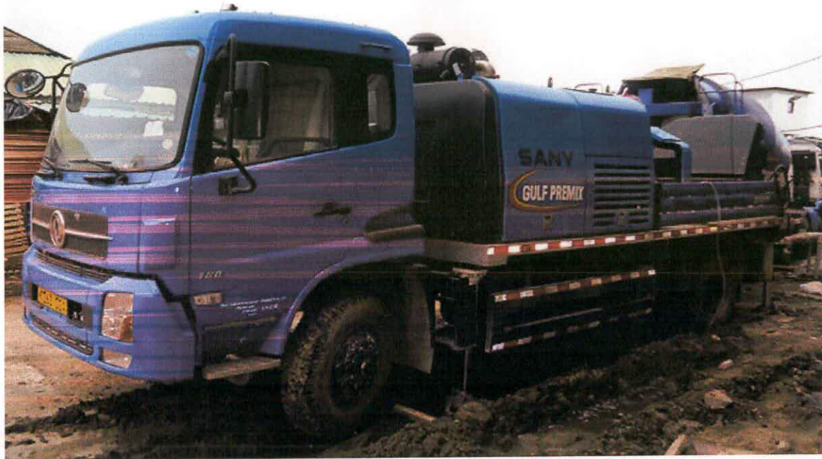
Truck-mounted concrete pump
