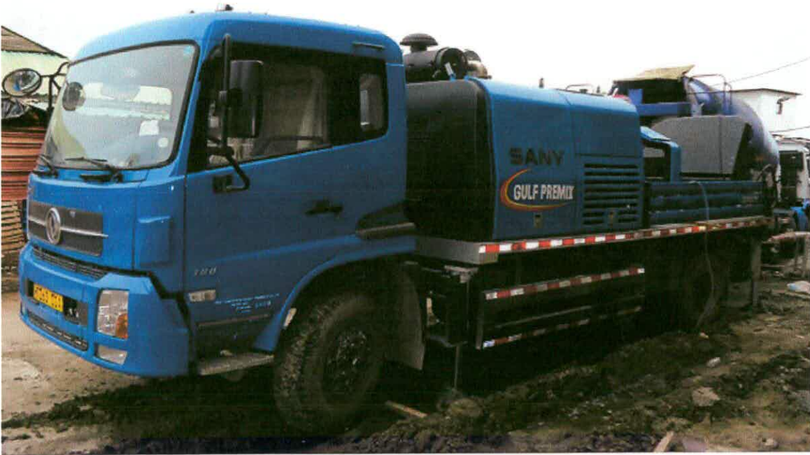
Truck-mounted concrete pump
