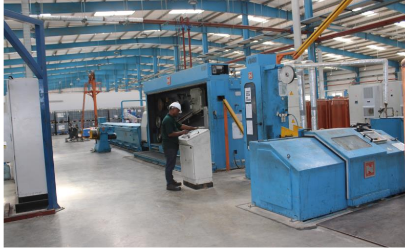
b) Heavy Drawing Copper M/C
