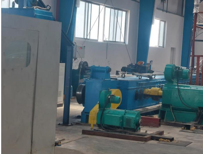
c) Heavy Drawing Aluminum M/C
