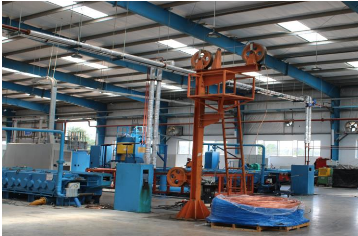
c) Heavy Drawing Copper M/C
