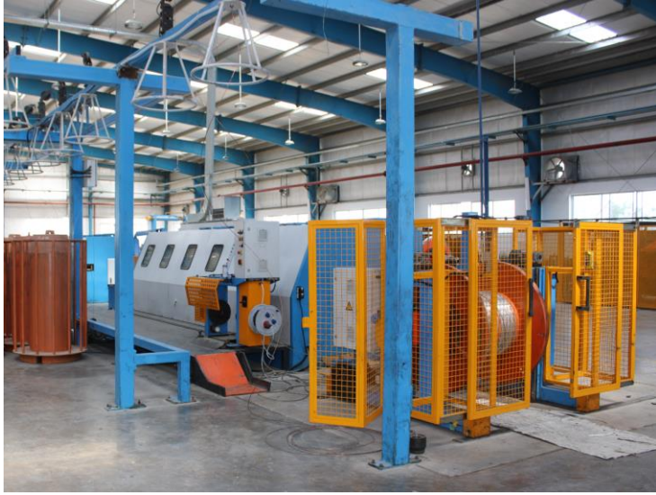
e) Double Twist 7 Wire M/C
