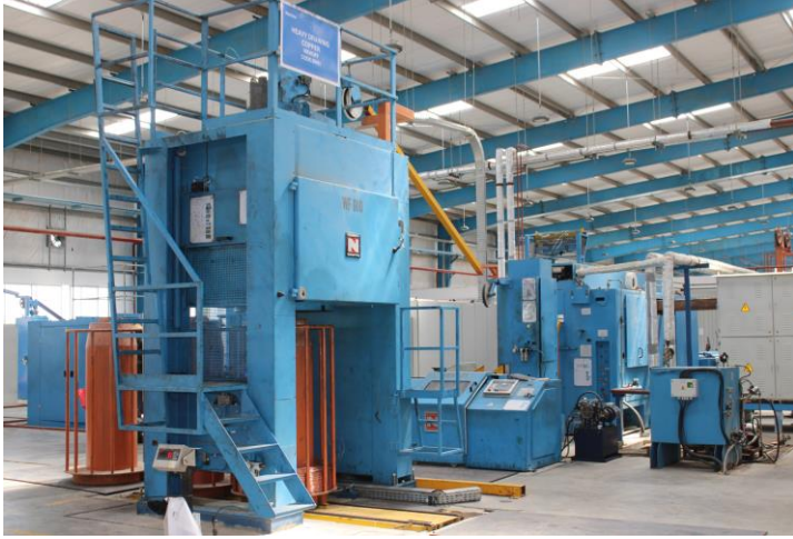
a) Heavy Drawing Copper M/C
