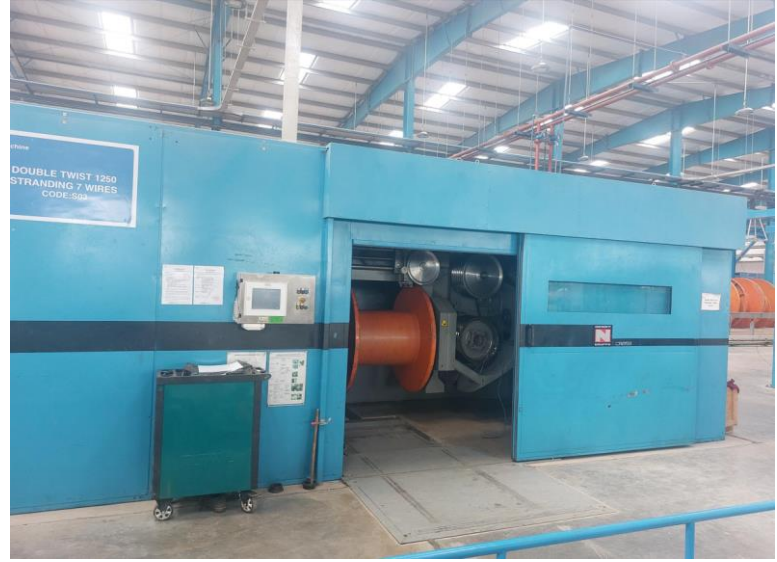
h) Tubular 7 wires stranding M/C
