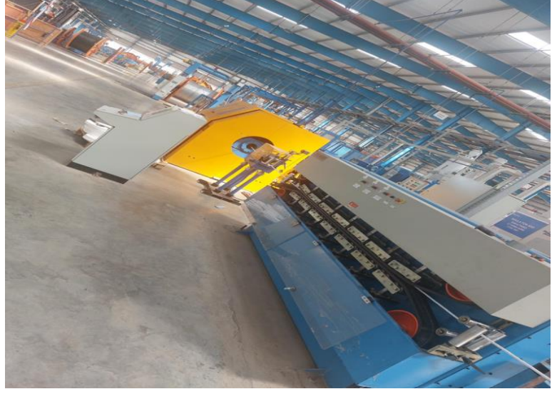
b) Tapping & Rewinding 2600 M/C
