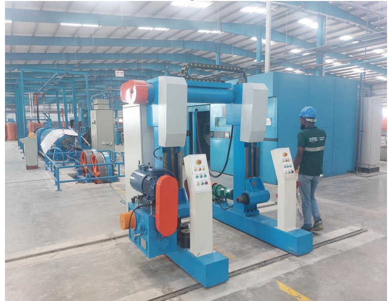
h) Tubular 7 wires stranding M/C
