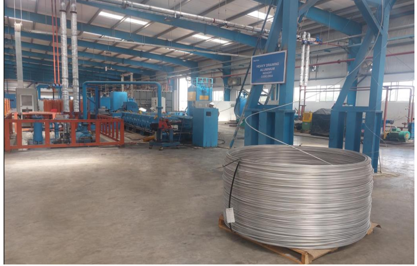
b) Heavy Drawing Aluminum M/C
