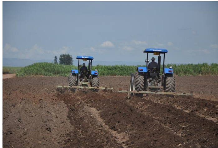
Step 9: Cane fields are ridged with ridging tractors to prepare for Cane planting process.
