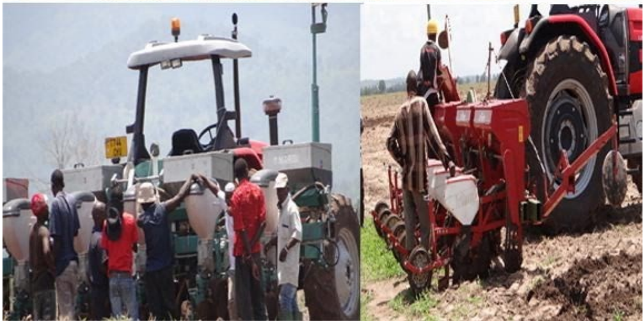
Planting with Pneumatic Vacuum precision planters and spraying with Boom Sprayers
