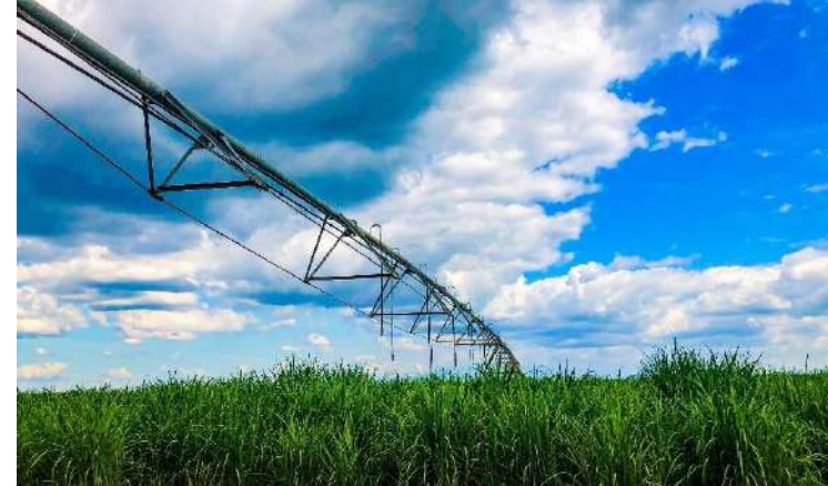
Overhead centre pivot system
