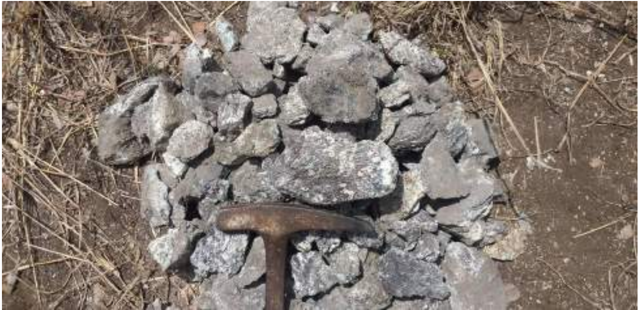
Plate 2.9: Weathered graphitic gneiss from trench number 09, Kwamsisi Graphite Project, Handeni 09 号沟的风化石墨片麻岩 (Source: Azustone Resources (T) Ltd, field work, 2022)
