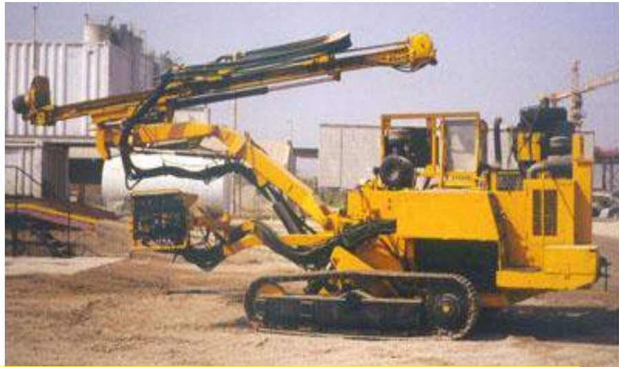
Plate 5.1: Example of a Mobile rock drill for Kwamsisi Graphite Project
