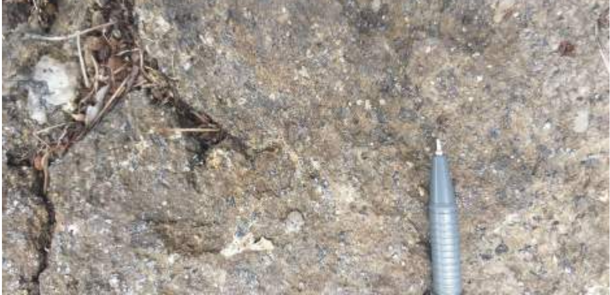
Plate 2.12: Coarse grained flake graphite in weathered crystalline limestone, Kwamsisi Graphite Project, Handeni 风化结晶石灰石中的粗粒片状石墨 (Source: Azustone Resources (T) Ltd, field work, 2022)
