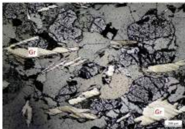
Fig.10: Microphotograph (10c) showing Graphite(Gr) under Reflected Light (RL) at 5X magnification objective.
