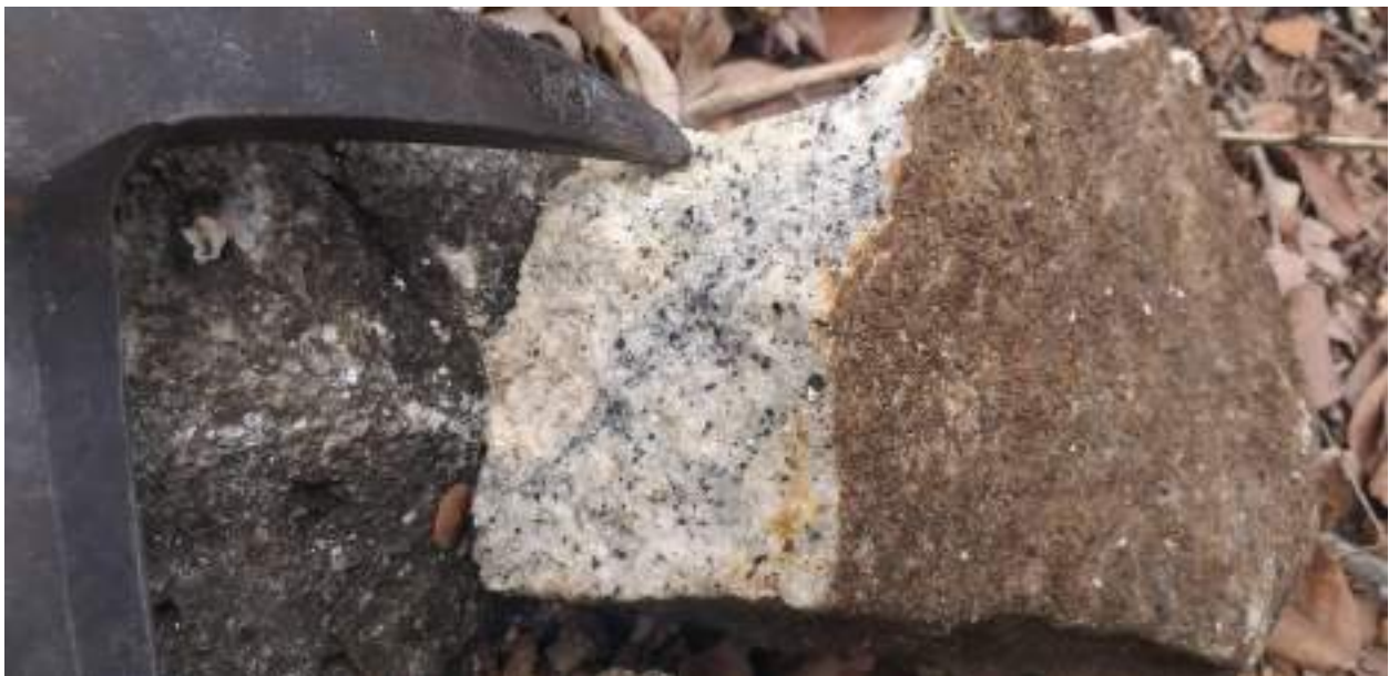
Plate 2.13: Low grade, coarse flake graphite mineralised in crystalline limestone Kwamsisi Graphite Project, Handeni 在结晶石灰石中矿化的低品位、粗片状石墨 (Source: Azustone Resources (T) Ltd, field work, 2022)
