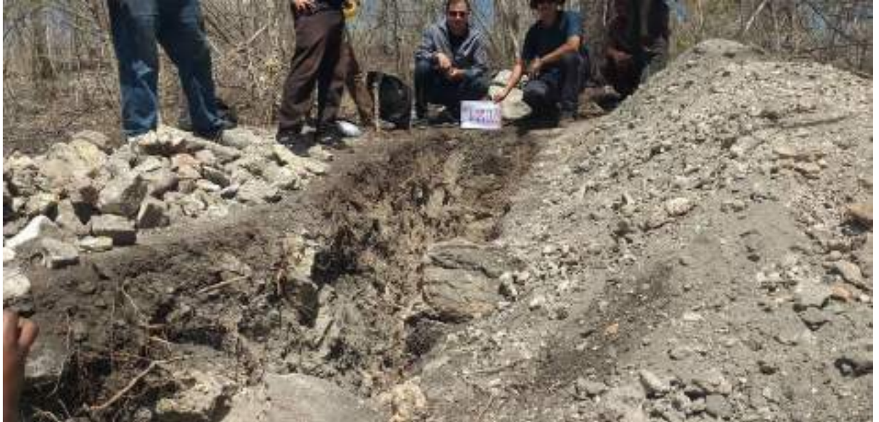
Plate 2.1: Trench Number 2 (TR02), crosscutting slightly weathered graphite mineralised gneissic rock, Kwamsisi Graphite Project, Handeni. 2号沟(TR02), 横切略风化的石墨矿化片麻岩
