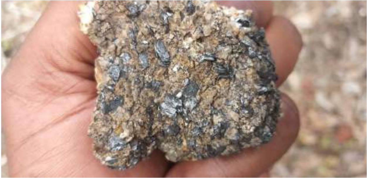
Plate 2.14: Verry coarse flake graphite from slightly weathered crystalline limestone, Kwamsisi Graphite Project, Handeni 由轻微风化的结晶石灰石中产生的非常粗糙的鳞片石墨 (Source: Azustone Resources (T) Ltd, field work, 2022)
