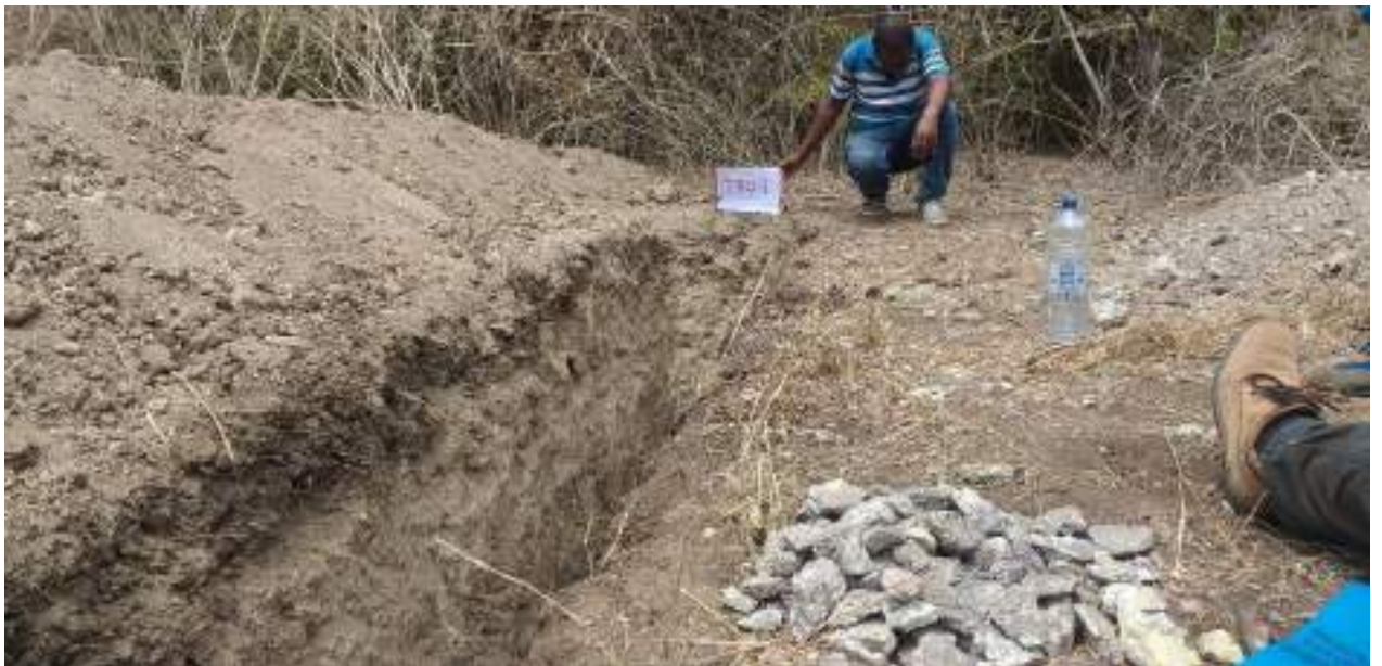
Plate 2.2: Trench Number 9 (TR09), crosscutting weathered graphite mineralised gneissic rock, Kwamsisi Graphite Project, Handeni. 9号沟(TR09), 横切风化石墨矿化片麻岩
