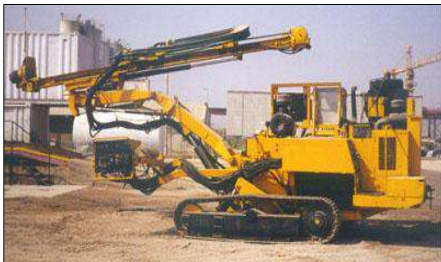
Plate 15.1: Example of a Mobile rock drill for Kwamsisi Graphite Project
