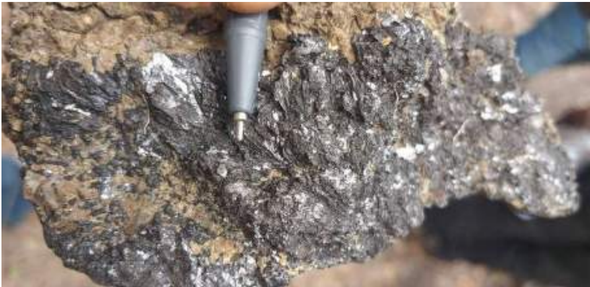
Plate 7.12: High grade, coarse flake graphite from slightly weathered crystalline limestone, Kwamsisi Graphite Project, Handeni (Source: Azustone Resources (T) Ltd, field work, 2022)
