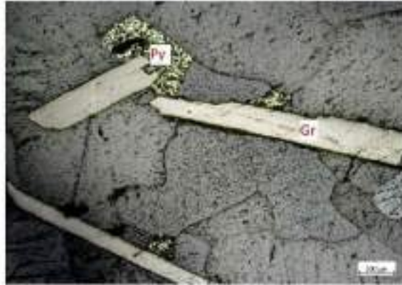
Fig.6:Microphotograph (6c) showing Graphite(Gr) and Pyrite(Py) under Reflected Light (RL) at 5X magnification objective.
