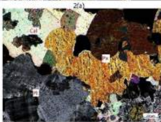
Fig.2: Microphotograph (2b) showing Calcite(Cal), Pyroxene (Px), Plagioclase(Pl) under Cross Polarised Light(XPL) at 5X magnification objective.
