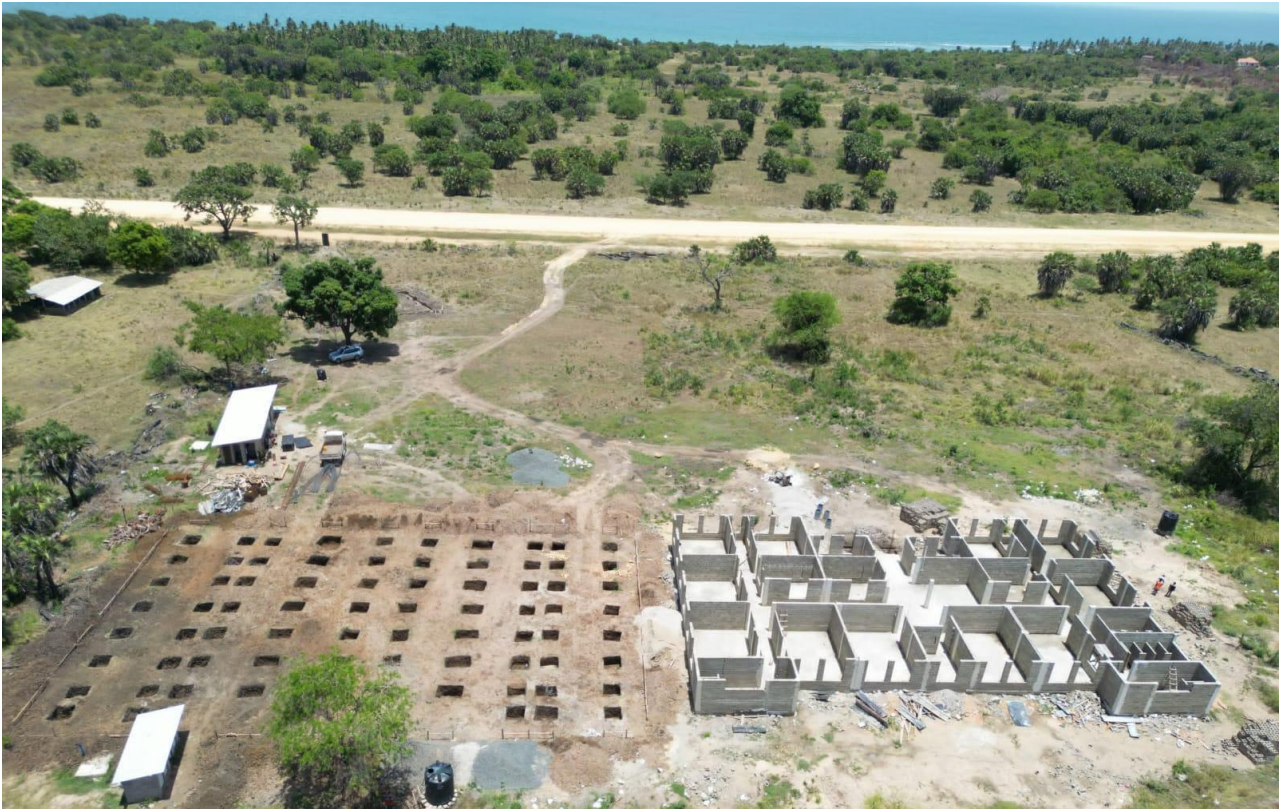
Figure 6. This picture shows the partially built pillars for the north wing in the foreground, and the west wing is in the background.
