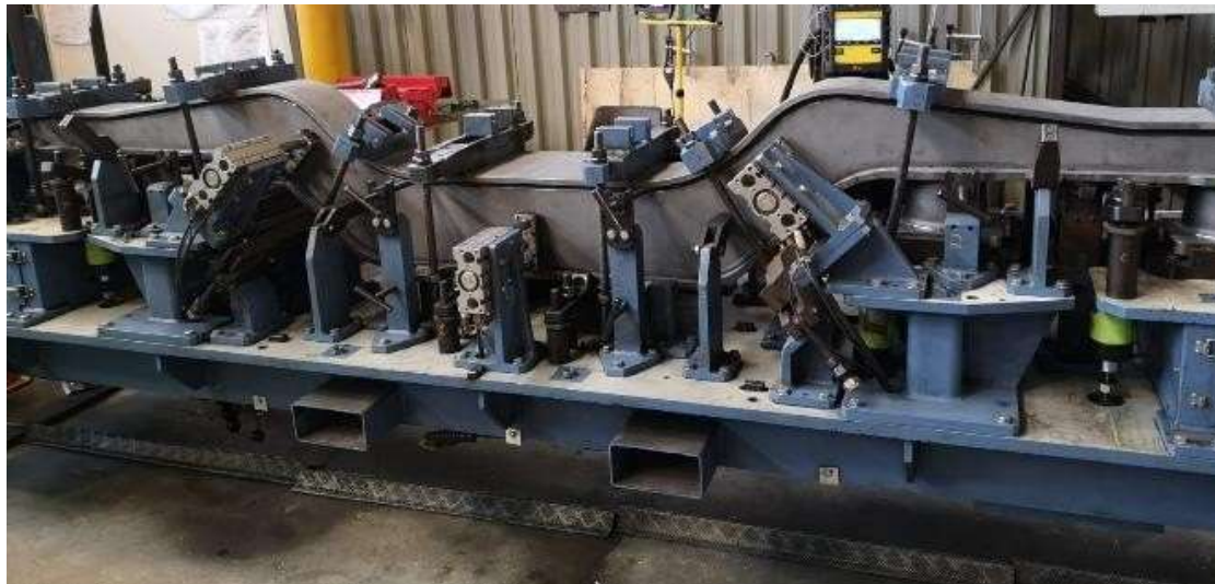
Bogie parts fitted to Alstom Ubunye jig
