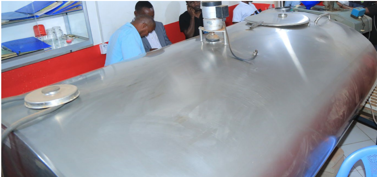
Figure 11: One of the Installed a 5000 ltrs cooler at the collection centre based at Kahama Fresh Dairy Farm at Kikulula
