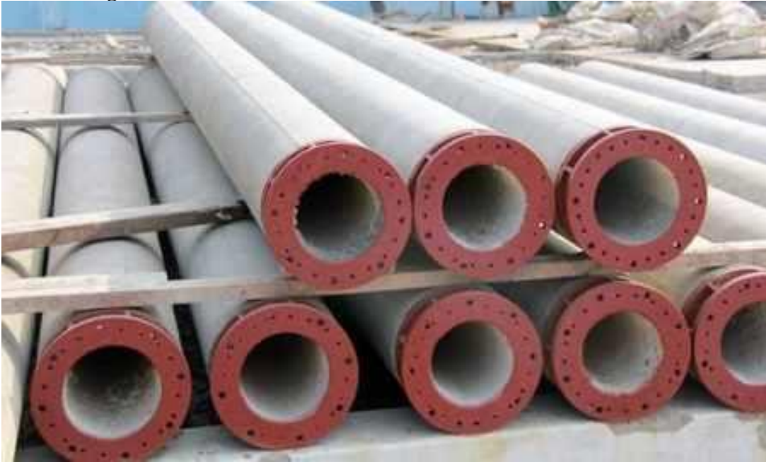
Figure 4: Mensel's Method Made Circular Hollow Concrete Poles
