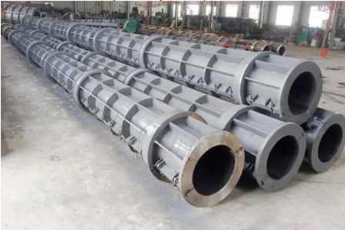
Figure 3: Long line Heavy Steel Molds
