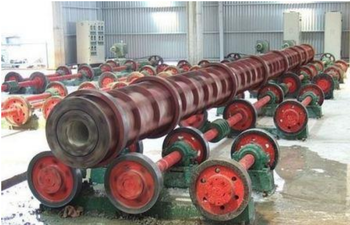
Figure 2: Centrifugal Casting Heavy Steel Molds
