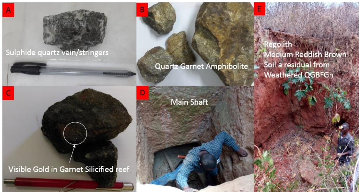
Figure 8. Mineralized potential units develop in the MGP as cropped from the deepest shaft within the applied mining licence area.
