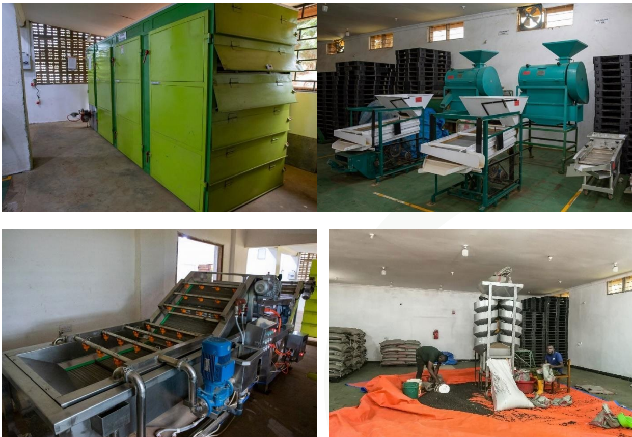
Clockwise from top left: Cardamom drier, Polishing (blue machines at back) and grading machines, Washer, Pepper spiral sorter
