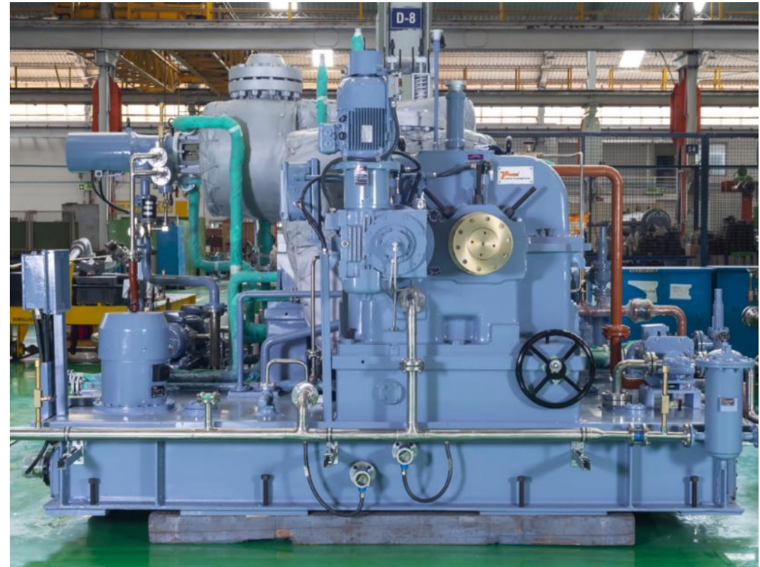
Extraction Condensing TA Set from Triveni
