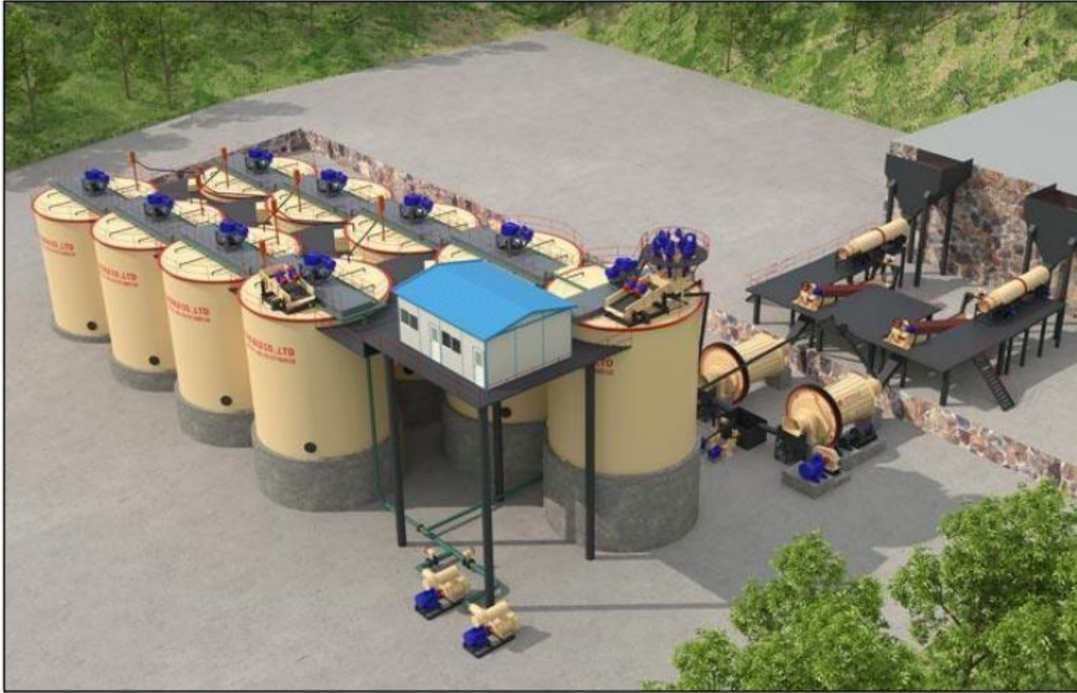
Figure 2: CIP or CIL schematic design diagram
