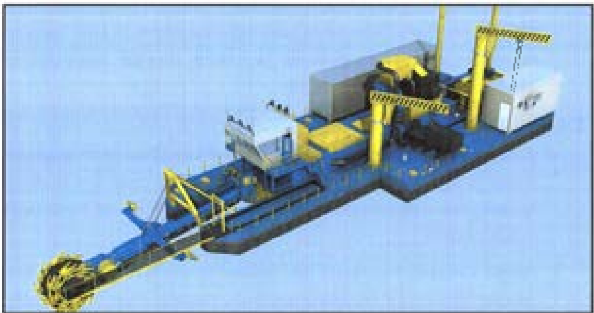
Figure 38: Cutter Suction Dredger
