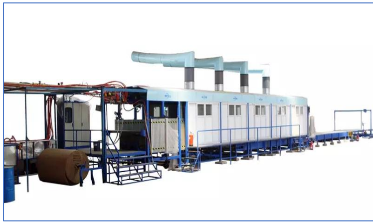
Step 2: Continuous Production Plant: Block Making
