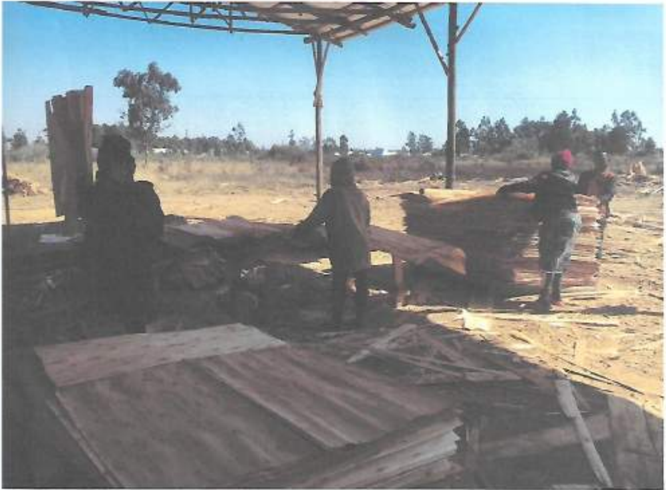
Figure 5-separation process of veneer and stick. Sources consultants, 2024
