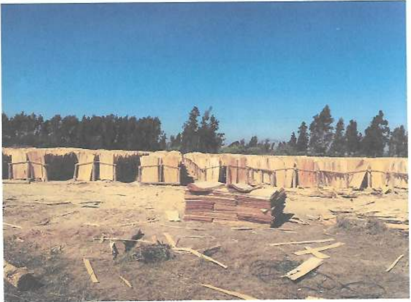
Figure 6 Drying process of wood veneer. Sources consultants, 2024
