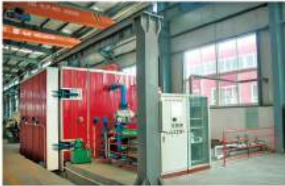
KDP-56W Vacuum Drying Equipment with Variable Pressure Method
