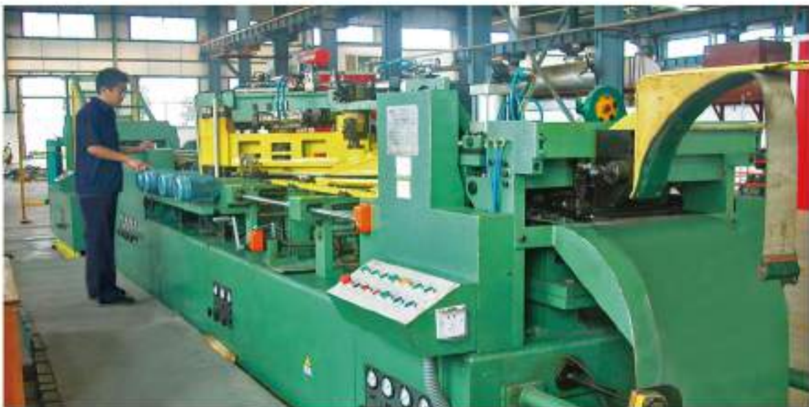
XBJ21-40 type silicon steel sheet(CNC)cross-cutting production line
