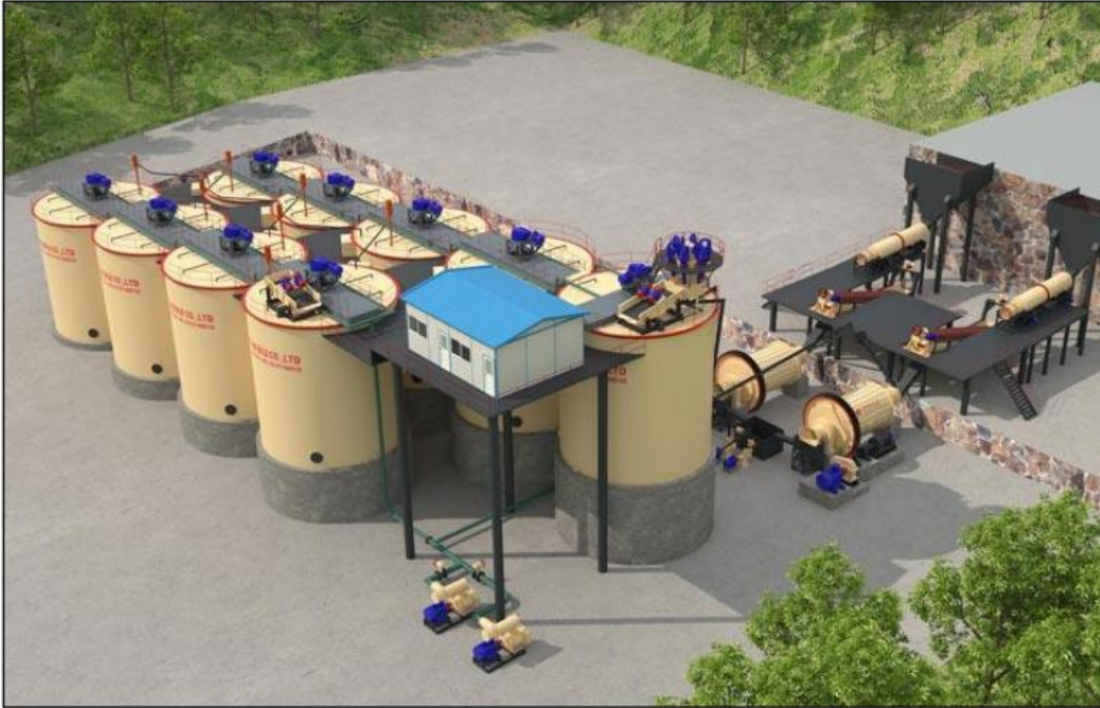
Figure 2: CIP or CIL schematic design diagram
