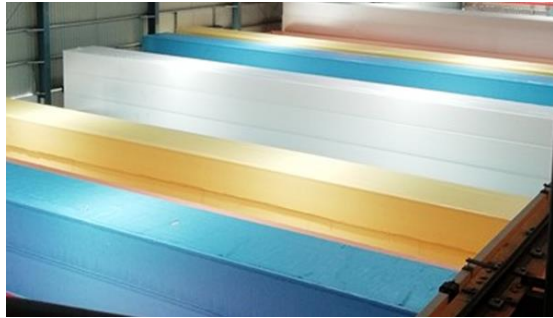
Step 4: Block Curing
