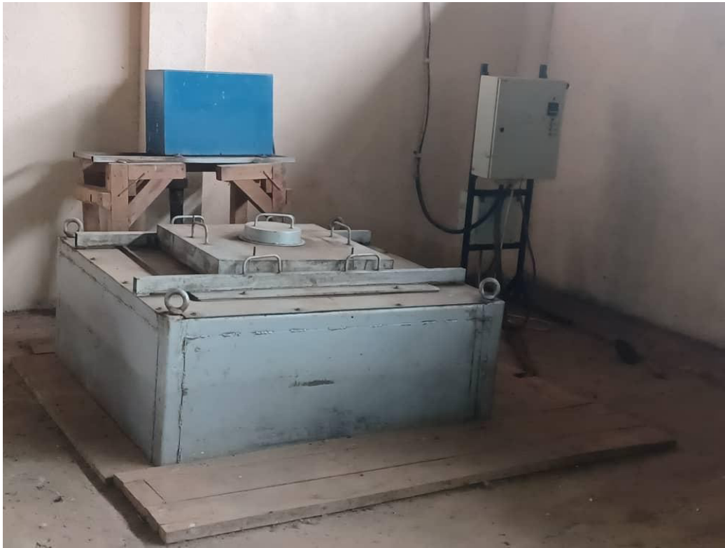
Figure 7. Tin Refining Equipment to Achieve 99% Purity
