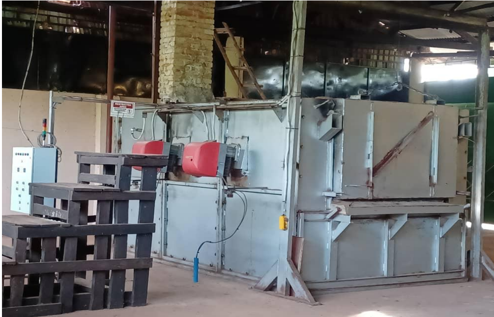
Figure 5. Large Melting Tank for Tin – Capable of Melting 3 tons of Tin at Once, Melting Tin Ore up to 85% Purity.
